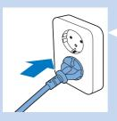
3 Put the plug in the wall outlet.
